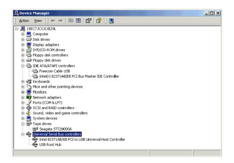
• If you are using the Travan 40GB tape drive, make sure that the Windows Device Manager shows a USB 2.0 Root Hub.
